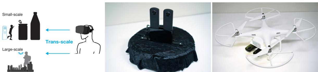
**Figure 1.** Left: Concept of a small-scale to large-scale trans-scale telexistence system. Middle: Our small-scale telexistence system comprising a controllable robot and omnidirectional cameras. Right: Our large-scale telexistence system comprising a drone.
